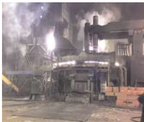
Figure 8.4 Image of operating electric arc furnace
